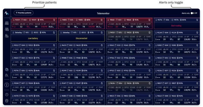
The Telemonitor screen is aimed for the use of telehealth centers and allows monitoring an entire department in a single view. This screen includes of a minimized version of a patient monitor for all patients assigned to the active department.
