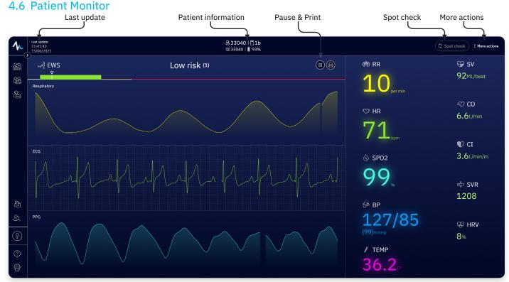
The **patient monitor screen** displays all vital signs measured in real time. When using a chest-monitor device, a one-lead ECG trace, a PPG, and respirations plots are displayed.
