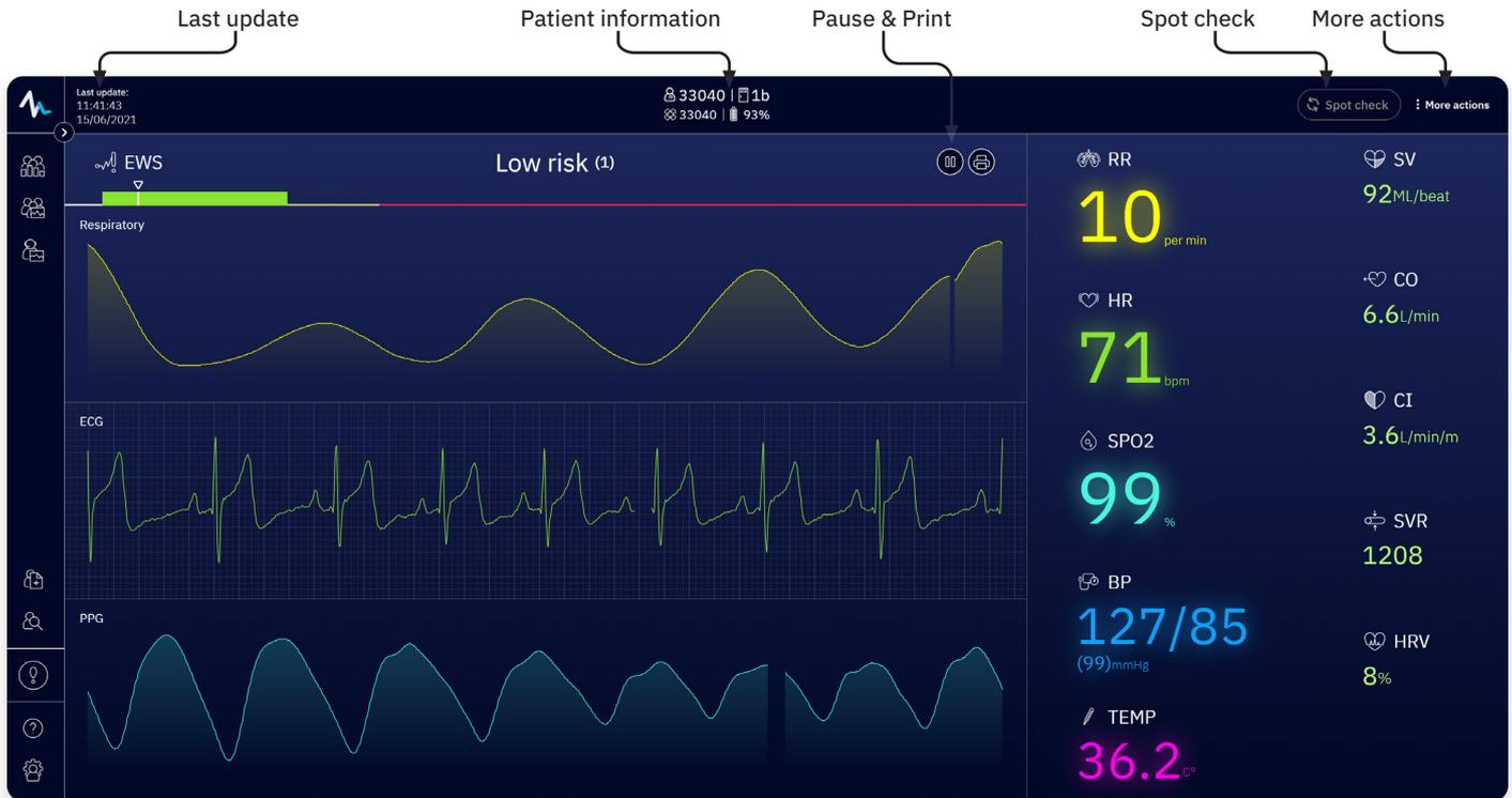
The **patient monitor screen** displays all vital signs measured in real time. When using a chest-monitor device, a one-lead ECG trace, a PPG, and respirations plots are displayed.
